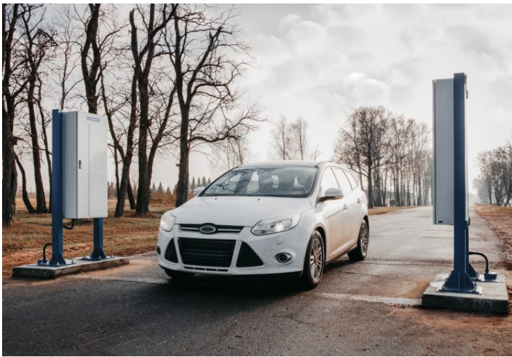
Version of vehicle radiation monitor with the following configuration: BDKG-19 (2 units), BDKN-05 (2 units)
