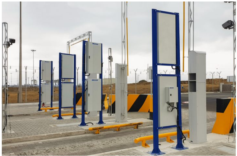
Version of vehicle radiation monitor with the following configuration: BDRM-05 (8 units), BDKN-05 (8 units)
